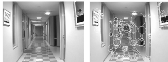
(a) A captured image in a corridor (b) Extracted features with SURF
